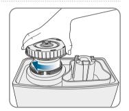
6 Fit the mist outlet in the water tank facing the front of the appliance for spraying.
